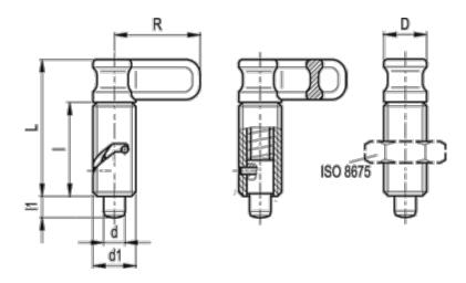
$\begin{array}{lll} D & = 16 \\ d - 0.02 - 0.04 & = 8 \\ d1 & = M16x1.5 \\ I1 & = 8 \\ L \ approx. & = 51 \\ I \ min & = 35 \\ R & = 32 \\ Spring \ pressure \ end \ (N) = 20 \end{array}$
